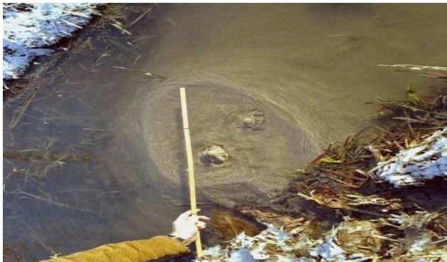
Figure 1-1 two sand boils as result of the piping process (Weijers, 2010)
