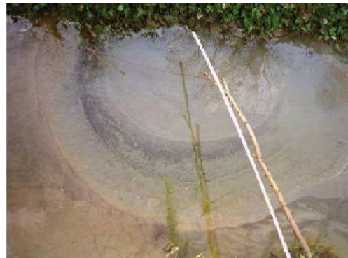
Figure 1-1 two sand boils as result of the piping process (Weijers, 2010)
